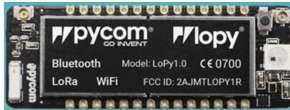
CPU: Espressif ESP32 chipset
