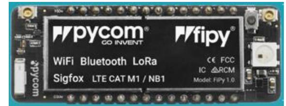
CPU: Espressif ESP 32 chipset
